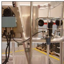
Wind speed control device, with alarm.
