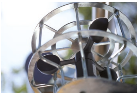
Anemometer for monitoring and warning that the maximum permissible wind speed (45km/h) has been reached
