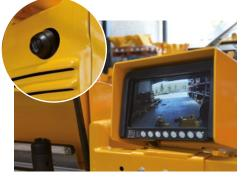
**Driving camera.** In order to improve driver visibility, it is possible to install an optional video camera and display to provide an improved view of the side opposite the aerial basket. This also facilitates alignment with the track when the platform enters the railway.
