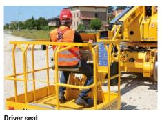
On request, a fold-down seat can be installed for the platform driver to make long transfers more comfortable.
