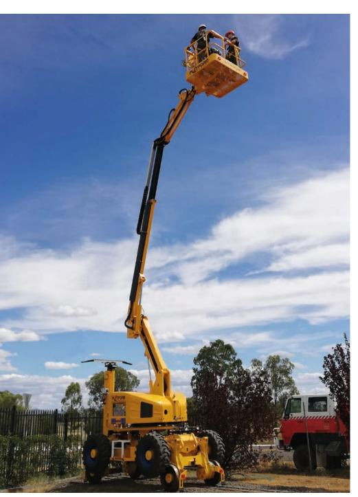
**The all-steel aerial basket** offers sufficient working space with the possibility of accommodating 3 people on board plus equipment (400kg).
