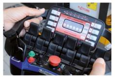
**Ergonomic and intuitive remote control** unit enable the easy movements of all machine functions.
