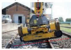
**The power** is delivered through a diesel endothermic engine of 10.5 KW power. On request it will also be possible to equip it for fully electric operation with lithium-ion batteries in order to make the equipment suitable for use in tunnels, subways and inside buildings such as hangars, stations, etc.
