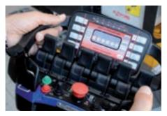
The machine can be operated using a remote control unit fitted on the basket or by the operator from the ground when there is no load in the basket.
