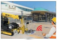
The remote control unit allows for easy operation of all machine functions. Operating the RR11T can almost feel like playing a game.
