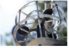
**Anemometer** (optional) For monitoring and warning that the maximum permissible wind speed (45km/h) has been reached.
