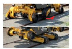
The 90° rotation of the tracks allows for an immediate switch from railway logistics to road logistics.
